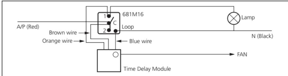
For applications where extract fan time delay is required for use without the light being included in the circuit, a momentary contact switch such as the 680M16P or 681M16PB may be used to replace the 681M16 switch module.
