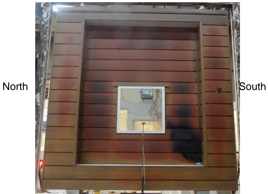
Figure A6.4: Exposed face of specimen at the end of the test
