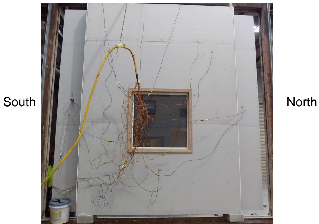
Figure A6.1: Unexposed face of specimen before commencement of the fire-resistance test
