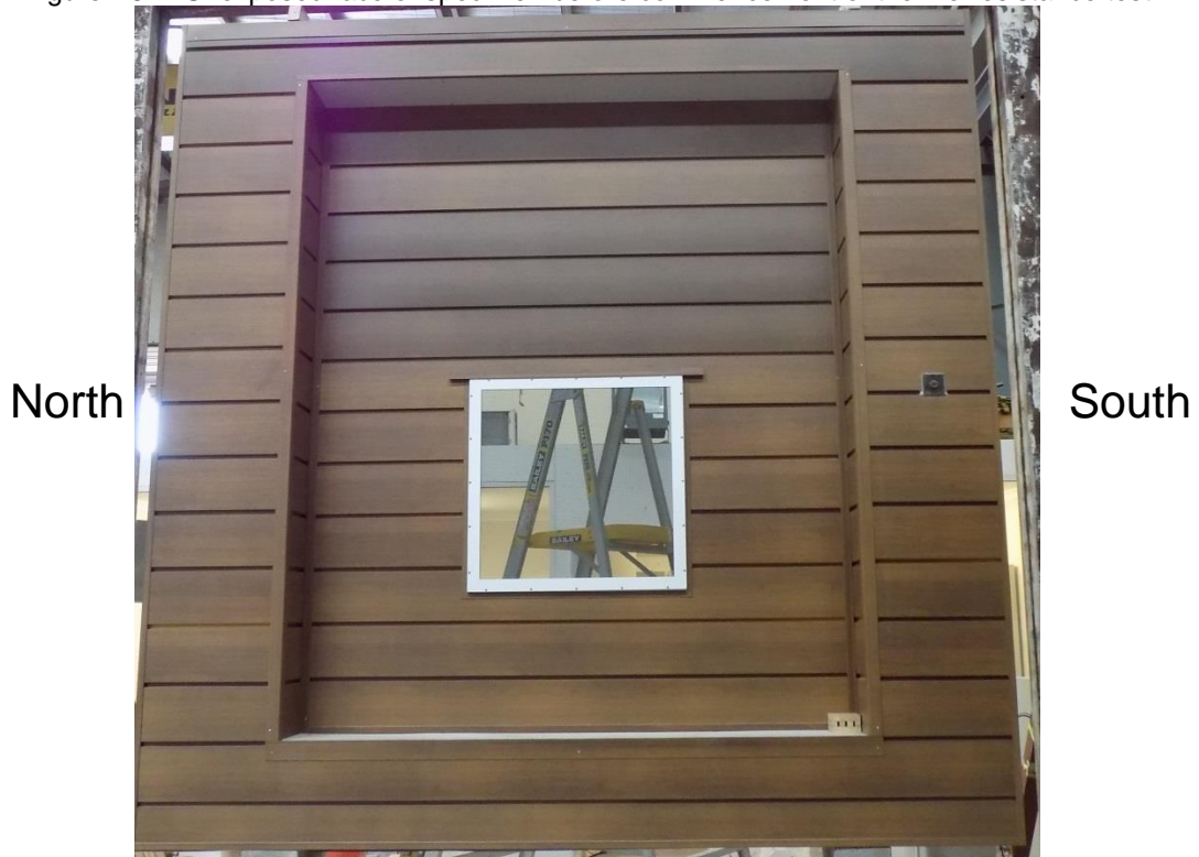
Figure A6.2: Exposed face of specimen before commencement of the fire-resistance test
