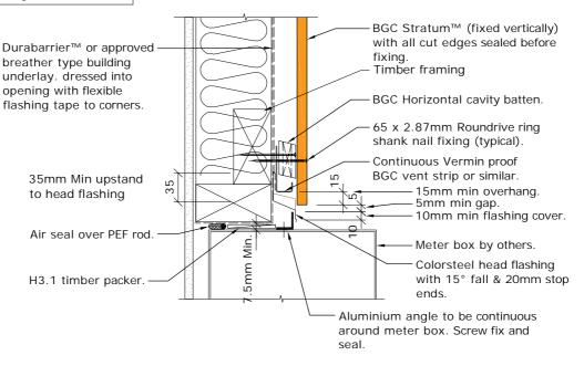
Note. Where  $\mathsf{Durabarrier}^\mathsf{TM}$  is used flashing tape must be applied to the entire opening
