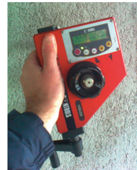
Assessing the render following the results of the pull-off test
