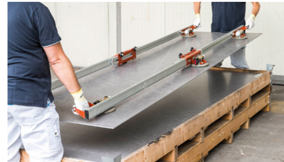
Moving slabs using equipment with special suckers
