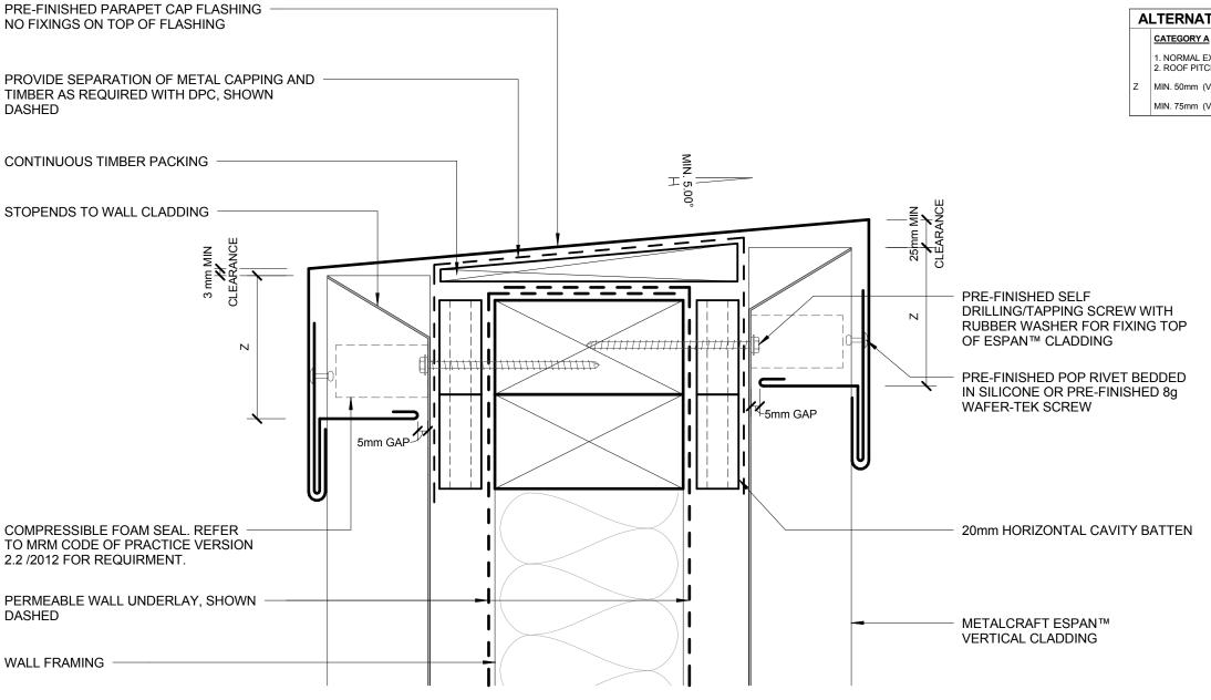
ACCEPTABLE SOLUTION AS PER E2/ASI SITUATION 1 SITUATION 3 1. ALL ROOF PITCHES IN VERY HIGH WIND ZONE 2. LOW, MEDIUM, HIGH WIND ZONES WHERE ROOF PITCH ≤ 10° 1. FOR ALL ROOF PITCHES IN EXTRA HIGH WIND ZONES 1. LOW, MEDIUM, HIGH WIND ZONES, WHERE ROOF PITCH ≥ 10° MIN. 50mm MIN. 70mm MIN. 90mm
