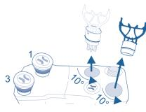
2. ▷ take out the inner valve insert with ball and the inner inlet insert. To do so, insert the special tool inside the groove, turn it anti-clockwise by 10° and pull it out
