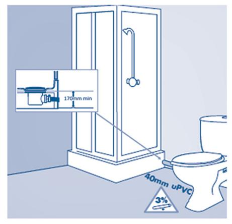
When connecting a shower to the **Sanimulti** the shower must be elevated to a height of no less than 170 mm from the shower grate to the base of the pump on finished floor level whilst maintaining 1:40 or 3% gradient on the shower waste fixture line.
