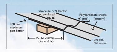
SPANS, OVERHANG AND END LAPS. Please refer to the Span Tables on the inside pages and do not exceed the measurements shown.
