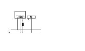
Standard operation parallel connection of max. 8 devices
