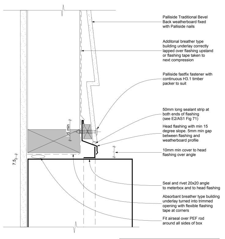
Fix angle and seal to all sides of box At sides and base cladding shall overlap by 10mm This detail is also suitable for other similar penetrations
