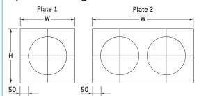
Plate constructed from aluminium sheet mounted in a Style No. 1 Frame surround, see page 51B. W and H dimensions listed are neck sizes.
