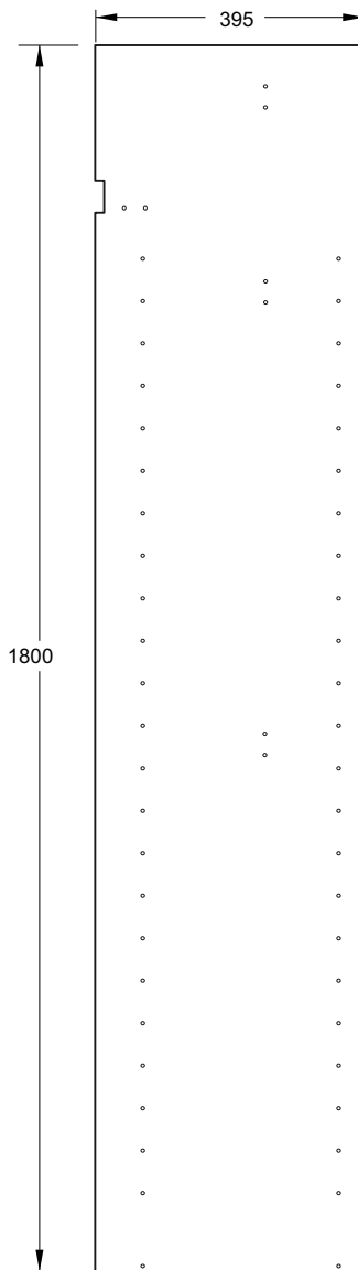
Drilling Layouts Adjustable Shelf Panel 1800mm x 395mm
