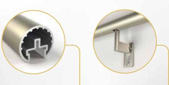
Patented twist-lock L-Brackets easily pivot for slopes and support over 225kgs each. Spacer Brackets included as required under the New Zealand Building Code.
