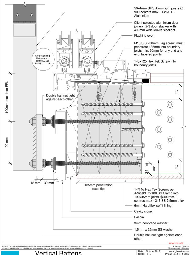
Vertical Battens 1300mm High Face Fixed into Timber
