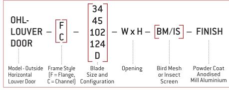
OHL-LOUVER DOORS are robustly constructed with Aluminium box section frames and extruded aluminium blades of the size and configuration required. High quality stainless steel hinges shall be used to support the relevant door loads. A 'High Quality' lock set and handle shall be provided as standard, as well as rubber seals to eliminate door rattle.
