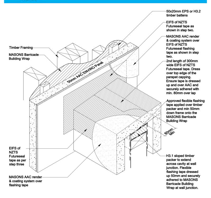
**PARAPET / HANDRAIL** TO WALL JUNCTION **ENVIRO Panel Capping** Step 4
