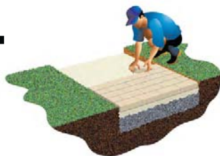
LAY THE PAVERS
