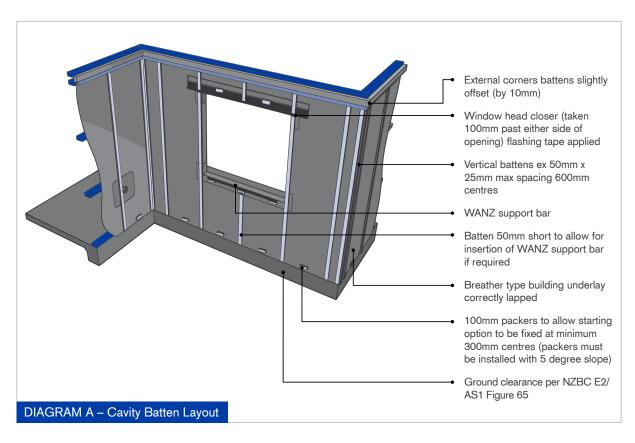
Structurally fixed batten equals MSG 8 framing grade H3.1 ex 50mm x 25mm fixed with 60mm x 2.8mm nails at 500mm centres (this allows for standard Palliside nails to be used instead of 60mm x 2.8mm).
