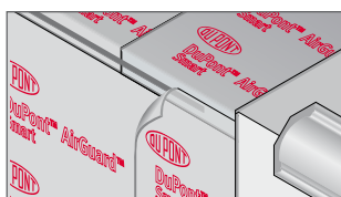
3 - Flat ceiling/wall junction
