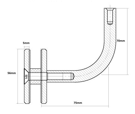
Visible 8mm countersunk screw fixing
