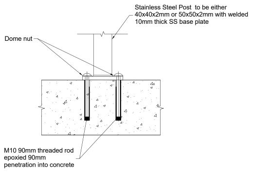
Stainless Steel Post for Nanorail® fixing applies to 40x40x2mm and 50x50x2mm posts
