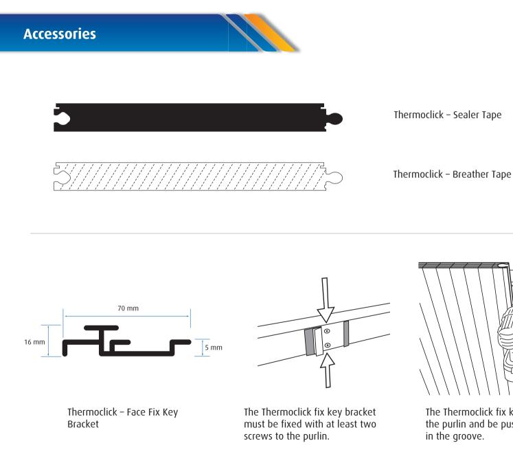
The Thermoclick fix key bracket must be positioned on the purlin and be pushed against the panel and located in the groove.
