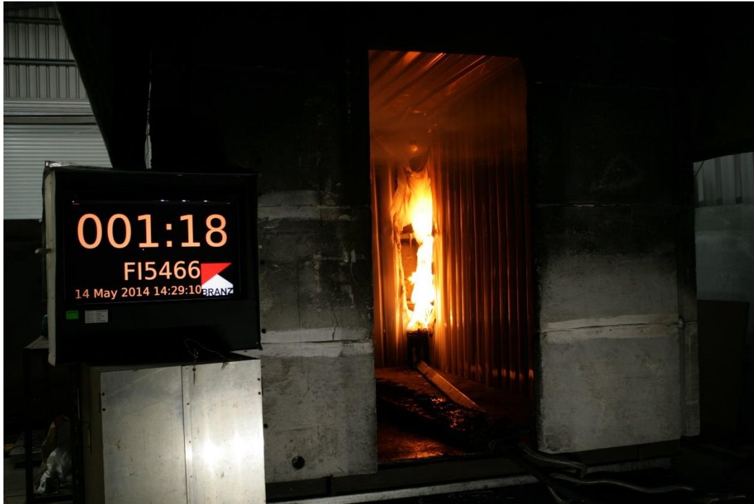
Photograph 6: Specimen at 129 seconds from start of test
