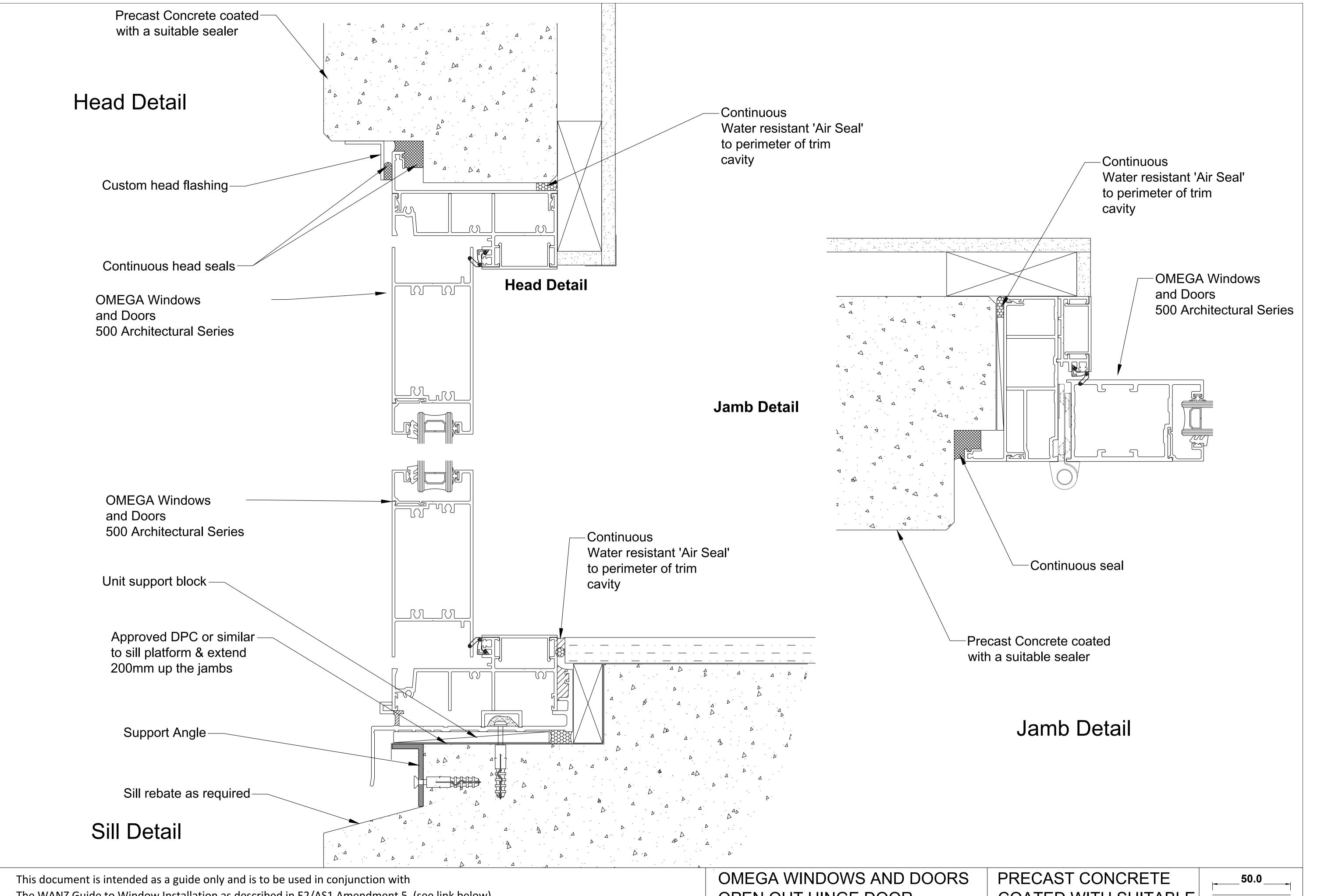
OPEN OUT HINGE DOOR 400 SERIES ARCHITECTURAL COATED WITH SUITABLE SEALER
