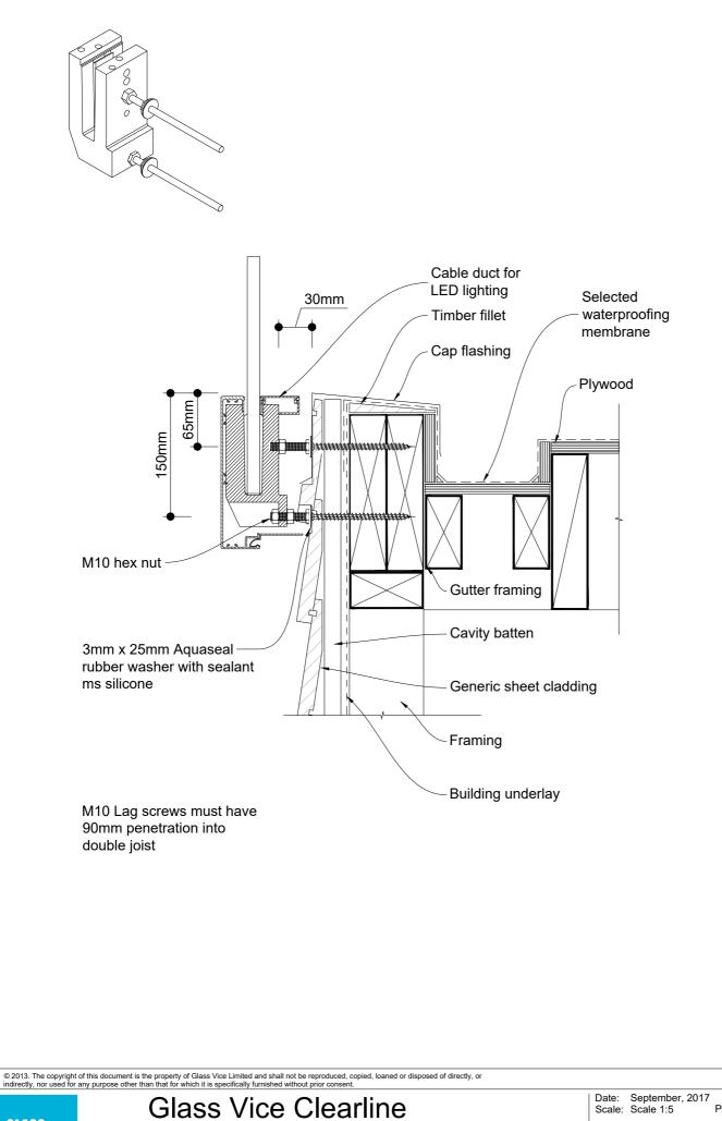
Panel Mounted Fixing Detail - 2 Point
