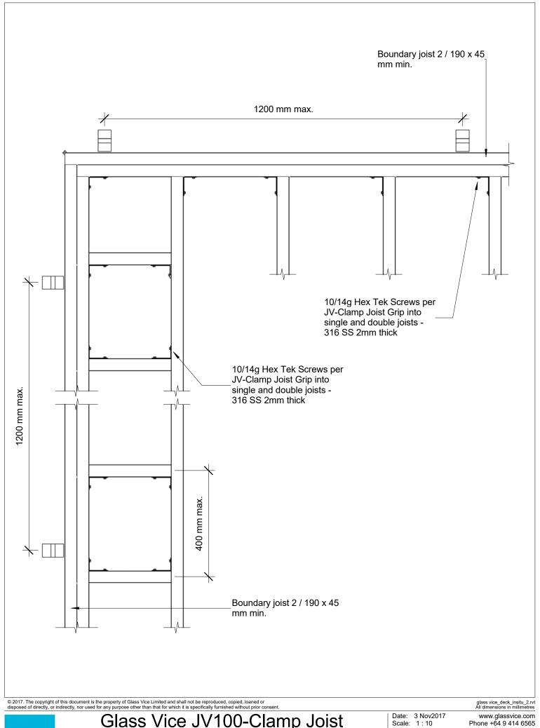
Glass Vice JV100-Clamp Joist Cantilever Deck - Framing 190mm
