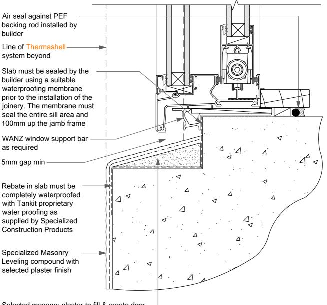
Selected masonry plaster to fill & create door sill with slop of 15 degrees min with selected finishing plaster to match cladding
