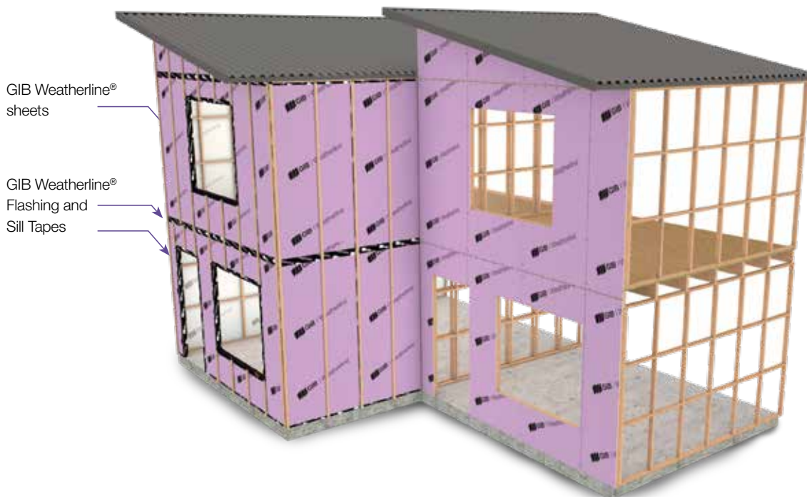
FIGURE 1: TYPICAL INSTALLATION OF GIB WEATHERLINE® SYSTEM
