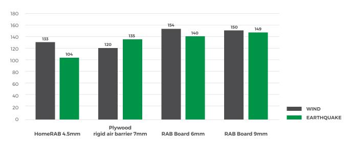
Bracing units per metre (length 1200mm)
