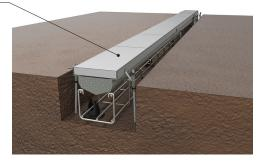
1st Pass: Concrete is poured to approx. 50mm above bottom of channel
