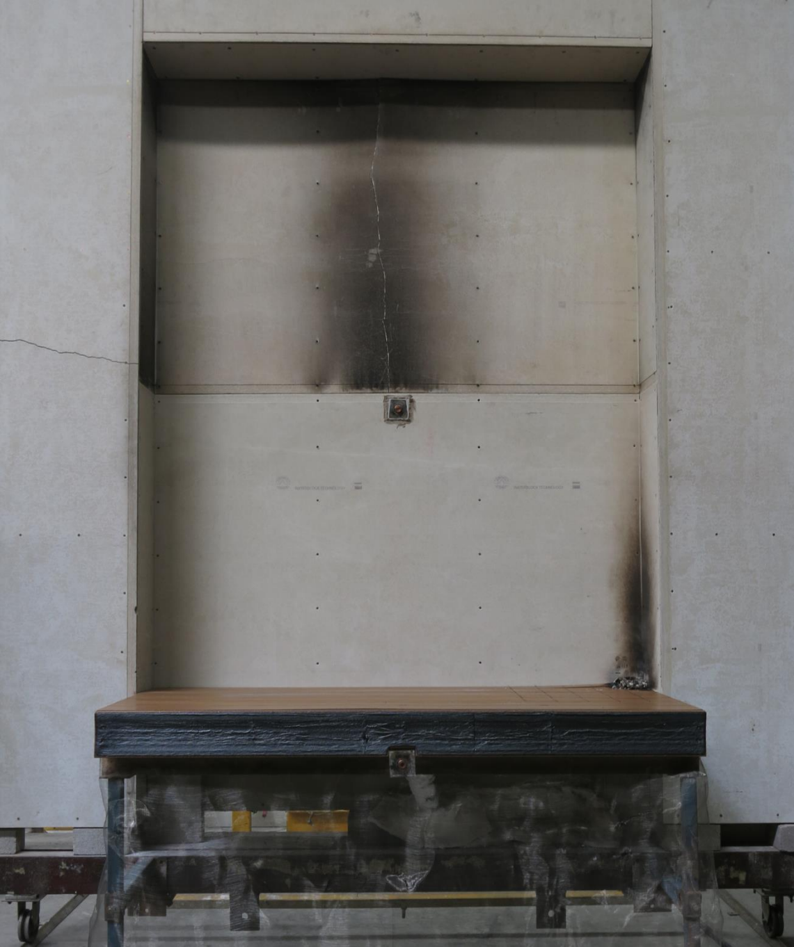
Figure A6.2: Exposed face of specimen at the end of the test
