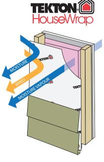
Tekton Wall Underlay is non-absorbent, breathable, fire retardant, flexible wall underlay.
