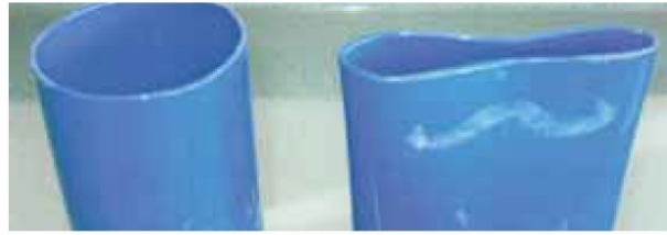
Abcite® coated pipe is scuffed but the film is not broken or chipped.
