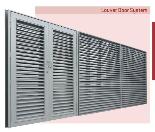
The louver doors are constructed with a rigid square frame to fix the hinges and the lock set to.\* The doors come standard with a High Quality lock set. The front of the door has a rubber seal on the closing face to eliminate door rattle. This also gives the door a positive closure feeling. The hinged posts of the doors have a security lip on the inside edge. This lip is there to prevent the doors being lifted out even if the hinge pins are removed.
