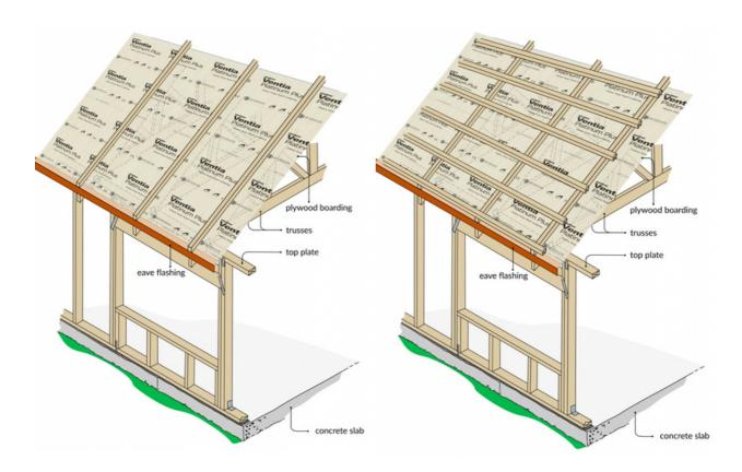
• Ventia Platinum Plus Underlay can be used on roofs with full plywood substrate e.g., bituminous shingle roofing systems.
