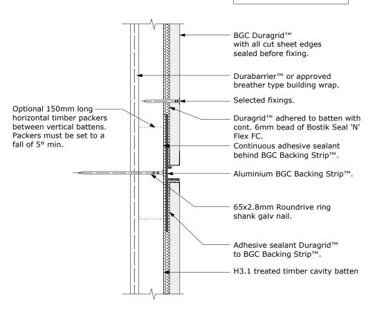
**NOTE**: ONLY suitable for up to 2 storeys in height. For cavities over 2 storeys in height, refer to D19
