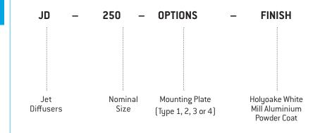
Circular Jet Diffusers shall be Holyoake Model JD constructed from spun aluminium cones. JD Jet Diffusers shall be capable of operating in either diffused, or jet air pattern configurations. The air patterns shall be achieved by rotating the cone assembly through 180 degrees. JD Jet Diffusers shall be complete with a mounting system suitable for wall, or ceiling applications.
