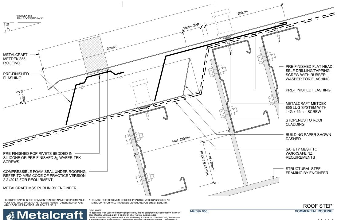
Details of the supporting mechanisms are indicative only. Compliance of the supporting mechanisms is the responsibility of the designer. Construction detail can vary for wall cladding. The underlay is detailed as a single line for simplicity and is indicative only. Building paper type and method of installation should comply with underlay manufacturers recommendations and NZBC regulations
