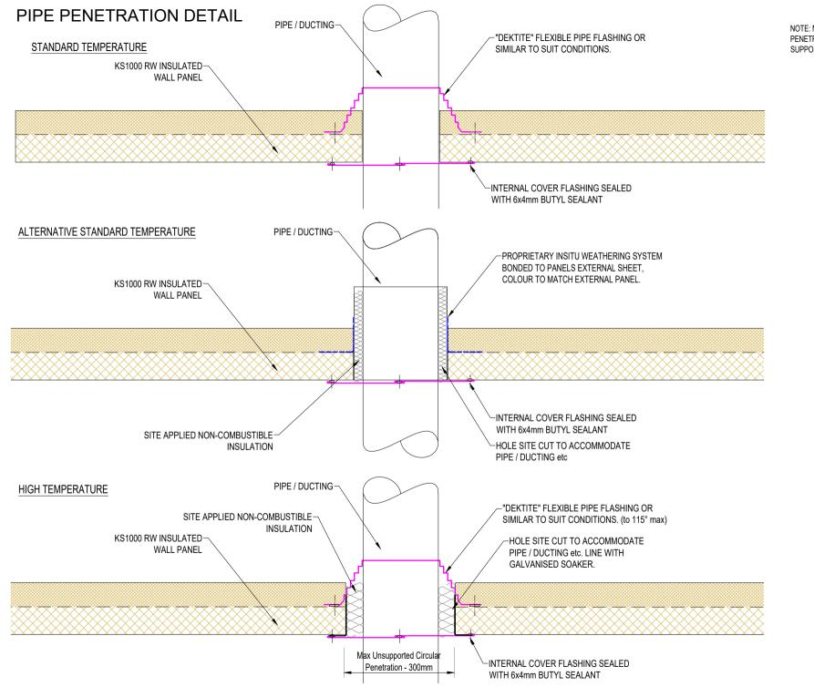
SYSTEM KS1000 RW\_STD WALL\_HORIZONTAL Q4\_2020 DESCRIPTION PIPE PENETRATION DETAIL APPROVED BY DATE REVISION JS 24.09.20 DRG REF: SCALE SHEET PAPER SIZE 1:5 1 of 1 RW\_HS\_15 A4 This document remains the property of Kingspan Ltd under copyright laws. Licence is granted to use this document and its contents in connection with Kingspan Ltd products only ©Kingspan Ltd DO NOT SCALE. IF IN DOUBT ASK
