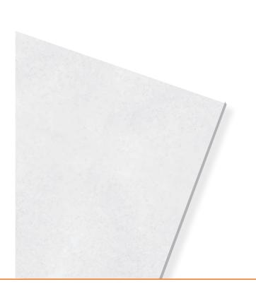
Thanks to its special composition, THERMATEX Aquatec shows moisture resistance of up to 100% RH. This means that even with a permanently high humidity and temperatures between 0 and 40°C the panel is inherently stable at all times. If necessary, THERMATEX Aquatec can be cleaned using water. Additionally, thanks to good sound absorption, the ceiling panel shows excellent acoustic features, which makes it a perfect solution for areas with strict hygiene requirements.
