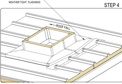
FIX AND SEAL AND SEAL-
