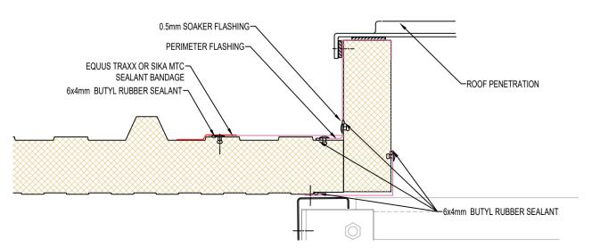
UPSTAND DIVERTER FLASHING (B) -
