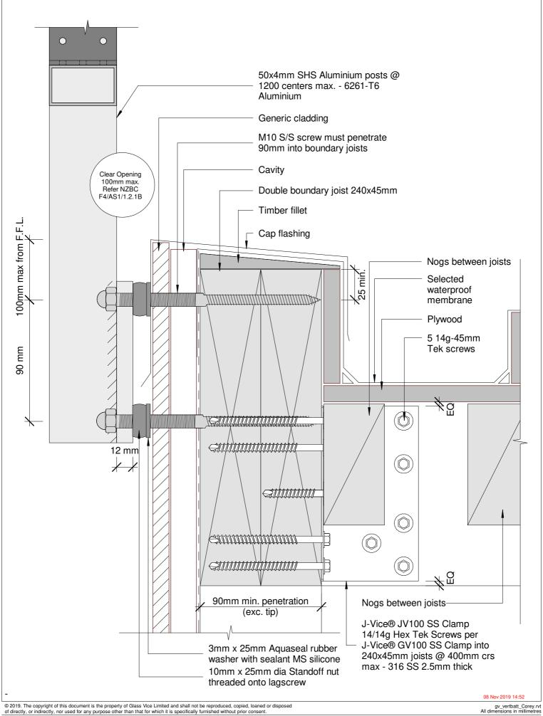
Vertical Battens 1100mm High Face Fixed into Timber Date: October 2019 Scale: 1:2 Issue 01
