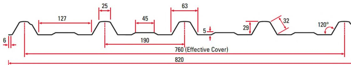
The scope of Acceptable Solution E2/AS1 for trapezoidal profile roofing is limited to those with a minimum crest height of 19 mm and 210 mm maximum between crests.
