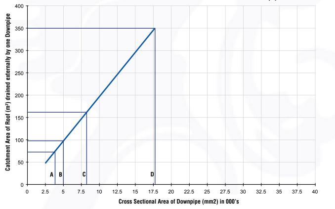
Note: The graph is based on a rainfall intensity of 100mm / hour and roof pitches less than 10 degrees. For more information on roof catchment areas and the effect of gutter cross sectional areas download the document on Roof Drainage
