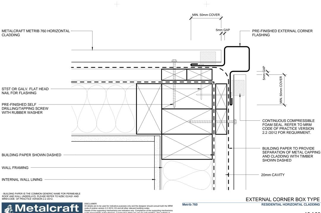
Details of the supporting mechanisms are indicative only. Compliance of the supporting mechanism is the responsibility of the designer. Construction detail can vary for wall cladding. The underlay is detailed as a single line for simplicity and is indicative only. Building paper type and method of installation should comply with underlay manufacturers recommendations and NZBC regulations.
