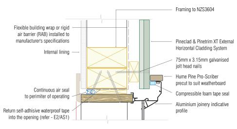
Hume Pine (NZ) Ltd Pineclad & Pinetrim XT Horizontal Weatherboard External Cladding Systems **Design & Installation Guide**
