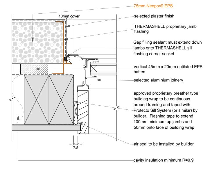
note: jambs and head flashing must be sealed or PVC welded where they intersect
