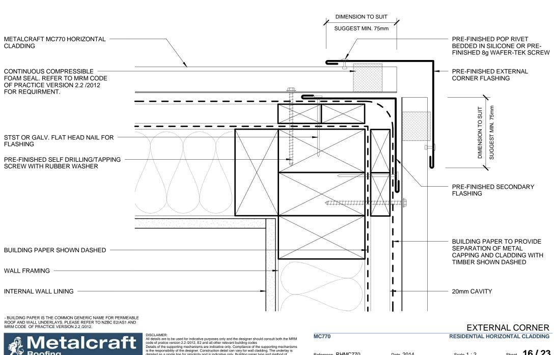
**Metalcraft** Roofing detailed as a single line for simplicity and is indicative only. Building paper type and method of installation should comply with underlay manufacturers recommendations and NZBC regulations.
