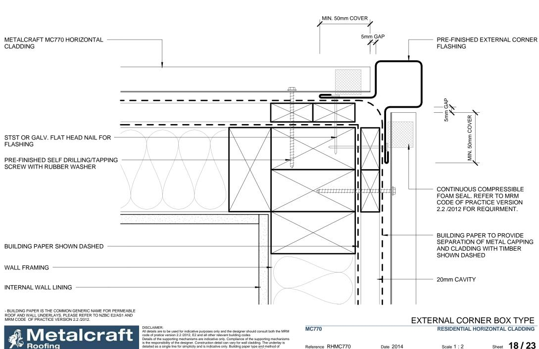
is the responsibility of the designer. Construction detail can vary for wall cladding. The underlay is detailed as a single line for simplicity and is indicative only. Building paper type and method of installation should comply with underlay manufacturers recommendations and NZBC regulations.
