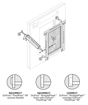
**NOTE:** Do not reverse shingle. DuPont<sup>™</sup> StraightFlash<sup>™</sup> must overlap DuPont<sup>™</sup> FlexWrap<sup>™</sup> NF and adhere to the substrate.
