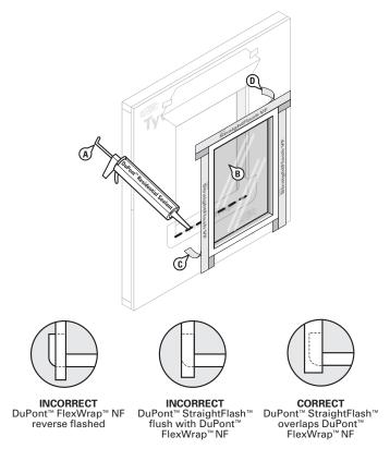
**NOTE:** Do not reverse shingle. DuPont<sup>™</sup> StraightFlash<sup>™</sup> must overlap DuPont<sup>™</sup> FlexWrap<sup>™</sup> NF and adhere to the substrate.
