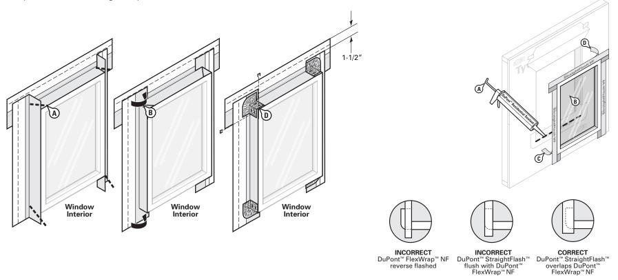
**NOTE:** Do not reverse shingle. DuPont<sup>™</sup> StraightFlash<sup>™</sup> must overlap DuPont<sup>™</sup> FlexWrap<sup>™</sup> NF and adhere to the substrate.
