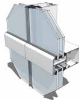
Drawings are of double glazed – captive. Please note: drawing(s) are not to scale. Structural glaze mullion only, no structural transom.
