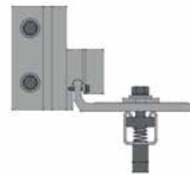
Curtain wall anchor (section)
