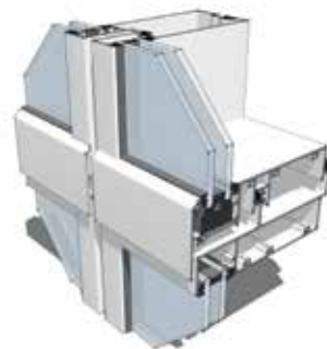
Drawings are of double glazed - captive. Please note: drawing(s) are not to scale.
