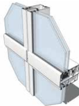
Drawings are of double glazed - captive. Please note: drawing(s) are not to scale.
