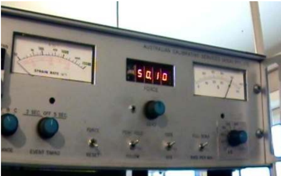
Testing of the Se015 anchor to 50.1kN.
