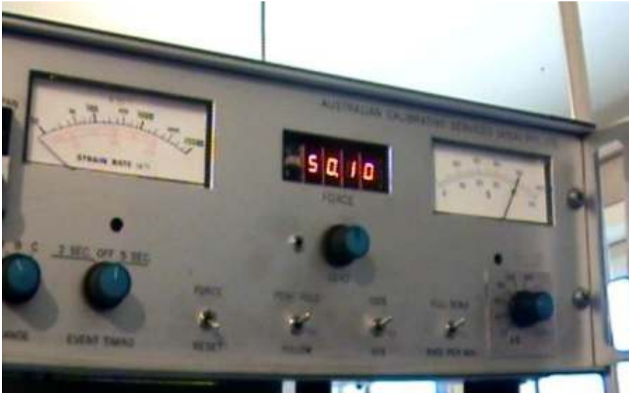
Testing of the SE015HP anchor to 50.1kN.
